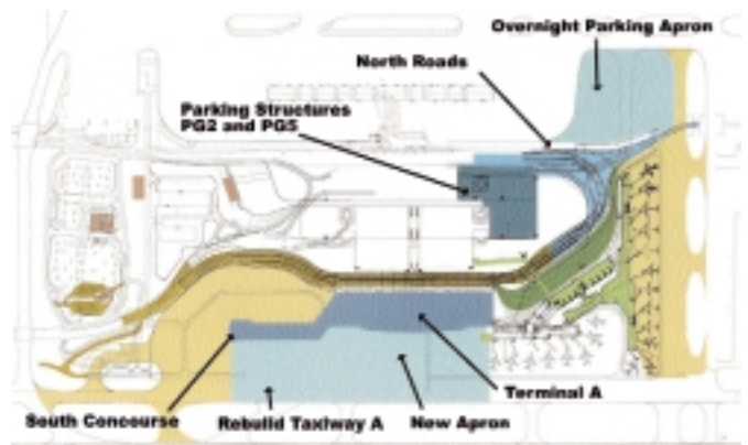
During the 30 months of Phase 2, passengers and airlines will use the interim terminal and Terminal A extension while the main portion of the existing Terminal A is demolished and rebuilt in the same location.
